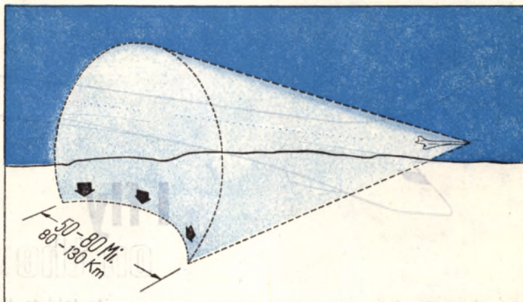
The "sonic boom" is heard along the flight path wherever the shock wave intersects with the ground
