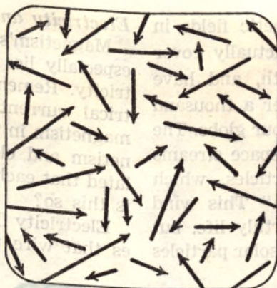
In nonmagnetized metals, small atomic groups are arranged with their magnetic poles situated at random
